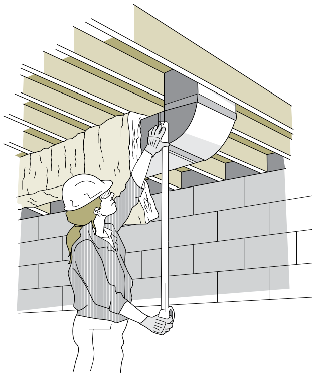
Figure 9-1 Taping an air duct
